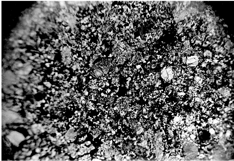
84: Plate 16: Figure B — The same, 10x. (The central squarish black patch and two large white ones easily compare with the same in Fig. A.) Concentric — radial shell-structure and spirodiscoid structure fairly clear.
