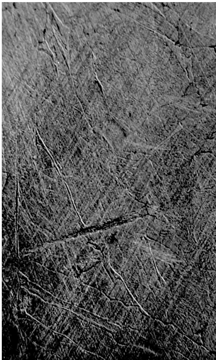
111: Plate 22: Figure C — Polished surface of Mazapil meteorite, 5x. The fine dotted or granular markings distinct from lines of the section or from cracks are here and there arranged in circular groups or defined curved bands.
