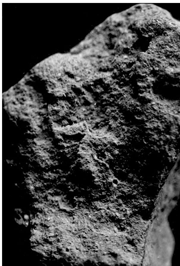
3: Plate 1: Figure 3 — Fragment of Red Clay, Challenger St. 165, 2600 fms., 5x and 8x, showing faint traces of nummulites. See Plate 21, Fig. C, D.
