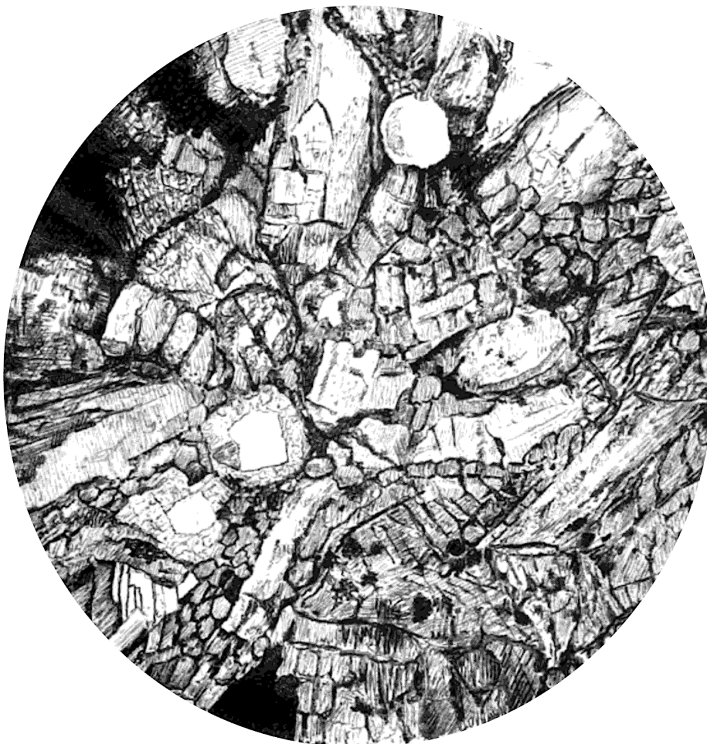
154: Table 2: Figure 10 — Thicker cut of the same artificial enstatite. Magnification 180.
