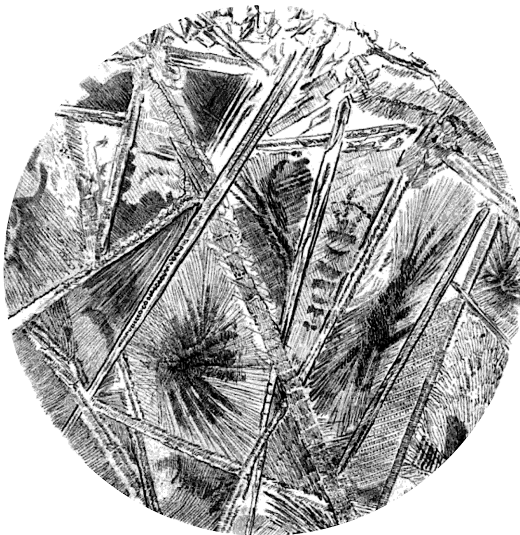
Figure 16: Thin section of enstatite produced by Mr. Daubrée by melting lherzolite with iron. Radiant fibers in fields circumscribed by crystalline rods. Magnification 50.
