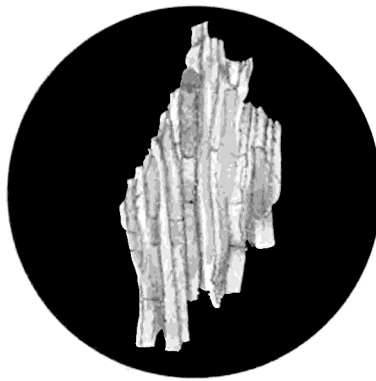
Figure 6: Splinter from Knyahinya, treated with potash, having a columnar and articulated disposition. Magnification 300. Crossed polars.
