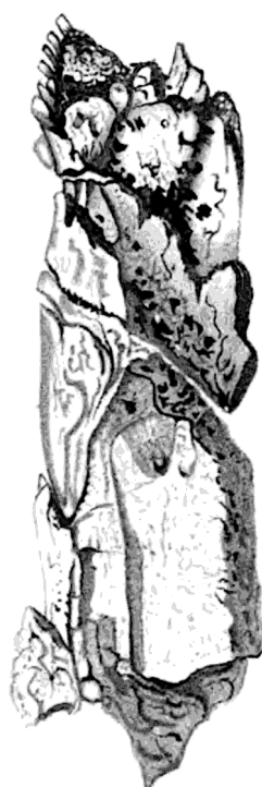
Figure 7: A crystal dislocated from Knyahinya. Magnification 300. The encrusting material penetrates everywhere and fills the small cavities of the surface.
