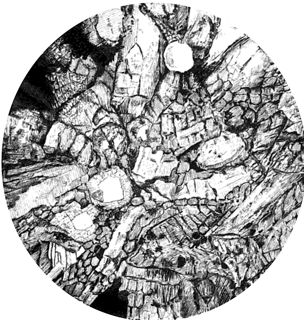
Figure 10: Table 2 — Thicker cut of the same artificial enstatite. Magnification 180.
